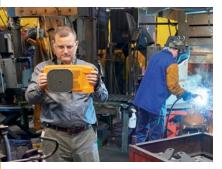
The ii900 Sonic Industrial Imager lets technicians see sound as they scan hoses, fittings and connections for leaks. Its built-in acoustic array of tiny sensitive microphones generates a spectrum of decibel levels per frequency. Based on this output, an algorithm calculates a sound image, known as a SoundMap, which is superimposed on a visual image. The SoundMap is automatically adapted, depending on the frequency level selected, so that background noise is filtered out.
