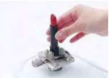
The test example of lipstick container turning force
