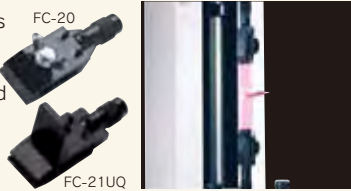
The test example of 180 degree peeling test of adhesive tapes with FC-21
