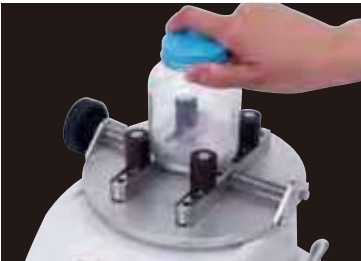
Screw cap opening torque test with DTXS.
