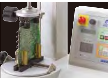
The test example of a circuit board twisting strength test with MTG.
