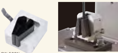
The test example of cable tension strength test with CW-500N..
