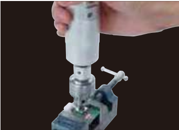
The test example of rotary switch click feeling test with HTGS.
