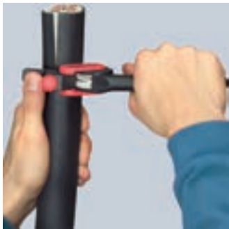
Turning the tool for circumferential cut
