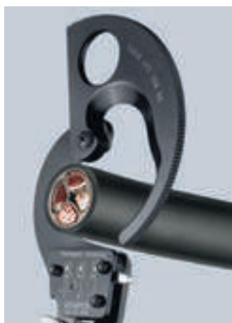
95 31 280: Large cutting capacity: maximum 52 mm dia. / 380 mm 2
