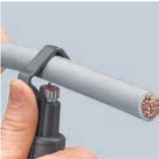
Setting the tool for circular cut
