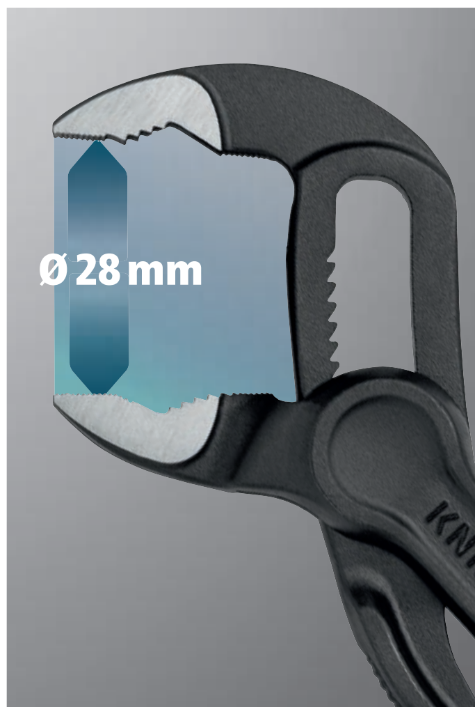
Naked truth: The grips are not coated to keep them as slim as possible. To ensure good grip, they are texturised on the outside
