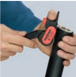
Setting the tool for longitudinal cut
