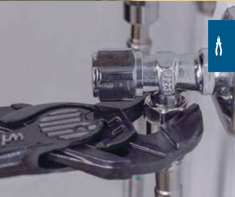
Quick fastening thanks to the ratchet function
