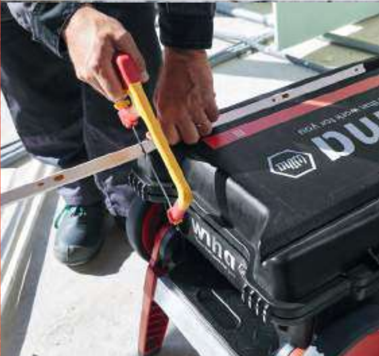
V-shaped notch with scale in the case lid
