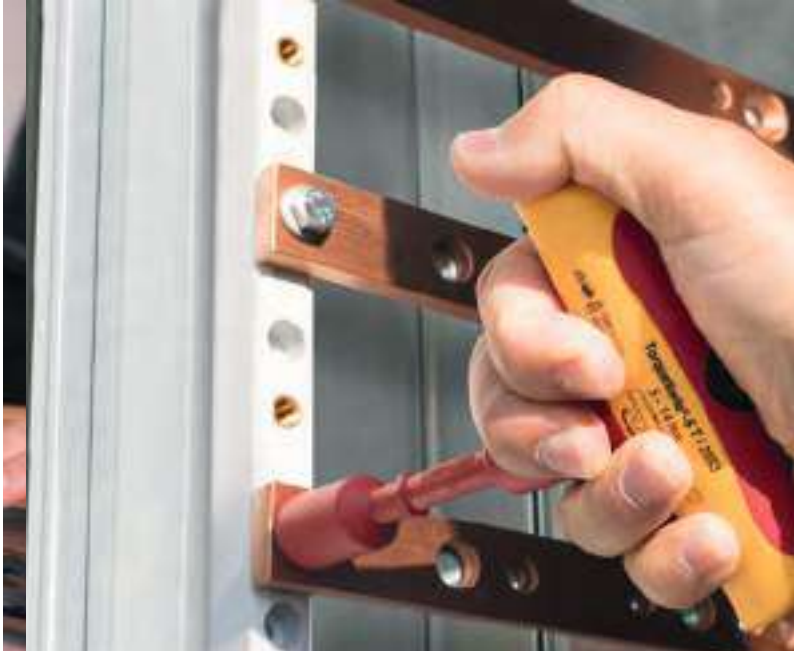
Lateral handle for high power transfer
