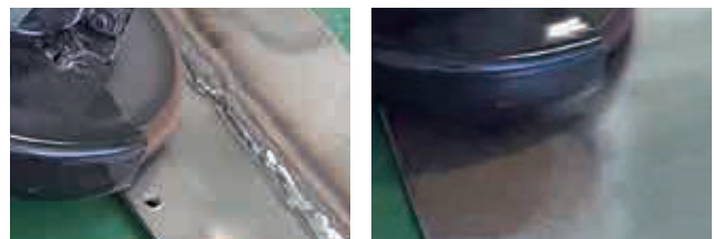
Removing blue weld discoloration Removing Rust
